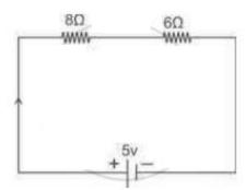
Calculate potential difference across the  $8\Omega$  resistor.
